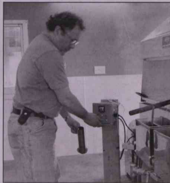
Using a new device that reads and evaluates the sugar content of the sap, Brian Benedict is able to tell the perfect temperature for boiling sap.
